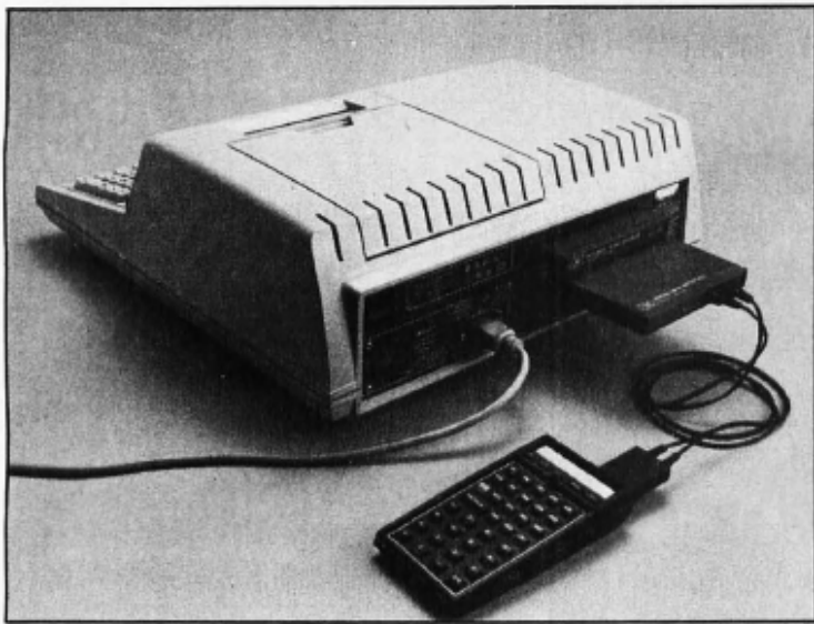
Photo 3: With the HP-41, HP82160A, HPIL Interface Module, HP-85, and HP82938A HPIL Interface Card, portable data collection, direct data transfer, and sophisticated data analysis are made easy.
