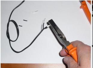
Fix the terminals on the wires
