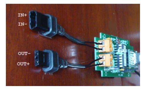
There are two ways to wire the HP-IL IN and OUT cables to the PIL-Box board:
