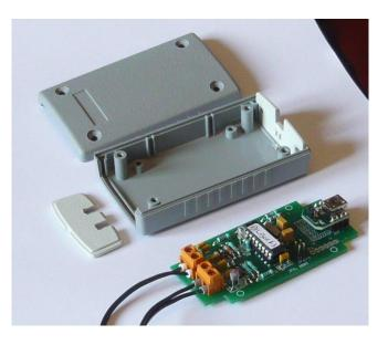
The top and bottom parts of the housing must be aligned, i.e. the 'notches' (the PILBox serial number is normally written on the top side 'notch') must be on the same side than the HPIL cable ouputs.
