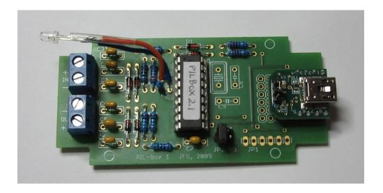
Remember: the LED cathode (shortest lead) is connected to the pad close to IC1 (blue wire here)
