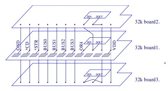
The 3 x 32k boards are chained by the DIN/DOUT pins of the 1LQ4(?) interface chip.
