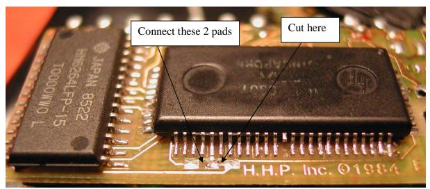
CAUTION: be sure to cut the short track between the 2 pads as indicated, otherwise a short-circuit will occur on the battery supply that may damage the small PCB tracks! Double check recommended!
