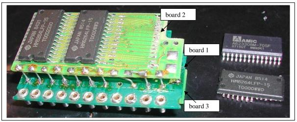
(picture taken while replacing a defective memory chip).
